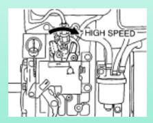
Once the engine is running, start the engine with the speed adjust lever at LOW speed and allow the engine to warm up. Increase the speed by moving the level to the right
