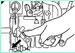
Before stopping the engine, reduce the speed of the motor for a few minutes before pressing the stop button to kill the engine
